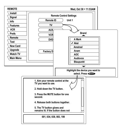
Device codes appear in the menu pane for the brand selected. Step-by-step onscreen help guides you through the procedure. Appendix B – *Manufacturers device control codes*, on page 43 also provides a complete list of device codes.
